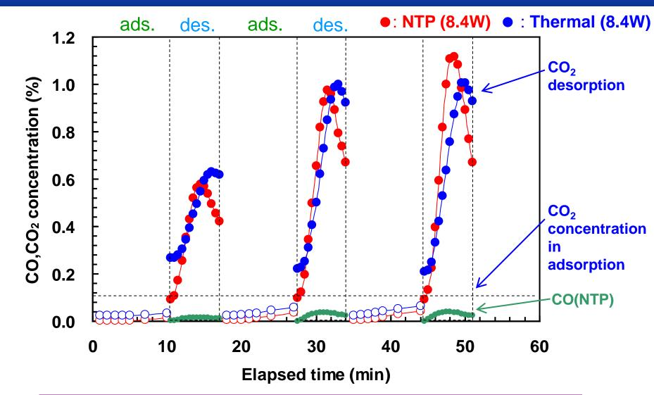
• For  $CO_2$  of 1000 ppm, the performance of NTP is higher.
