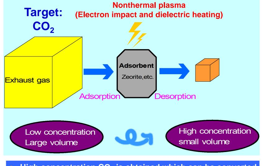
High concentration CO<sub>2</sub> is obtained which can be converted to CO with higher energy efficiency.
