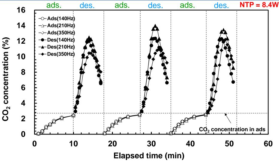
CO<sub>2</sub> desorption increases with increase in the frequency.
