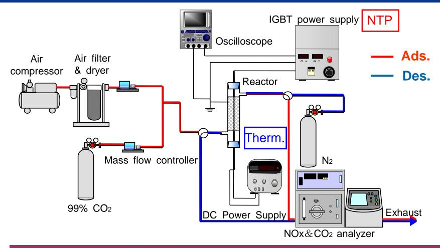
Adsorption: MS-13X (2mm, 12 g),  $CO_2 = 2.75\%$ , Q = 4.0 L/min, t = 10 min Desorption: flow rate = 0.5 L/min, t = 7 min, Input power = 8.4 W (NTP: IGBT f = 210 Hz or thermal heater )
