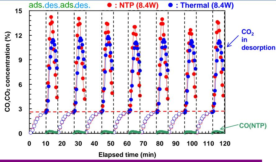
After 7 repeated adsorption/desorption, they reach the steady state.
